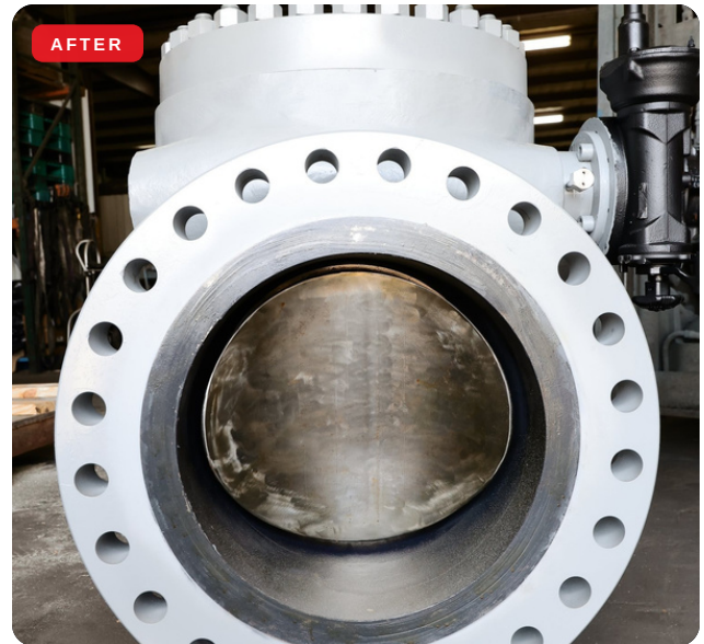
The finished valve, bore and seat machined and the flange face refaced, ready for a continuous pig path.
