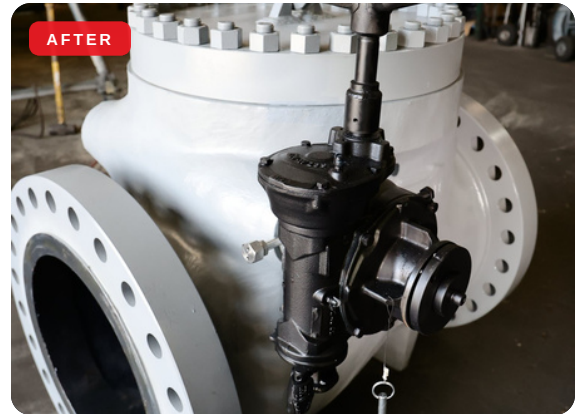
The finished valve with its gear operator, check and seal functions retained.
