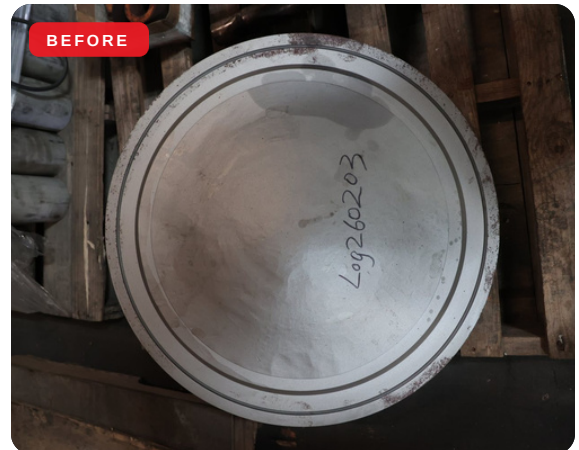
The valve's original clapper at the start of the project, before the conduit guide was engineered onto it.
