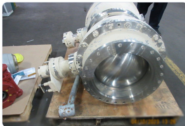
The rebuilt cryogenic valve, bore and seat finished to a zero-leakage standard.
