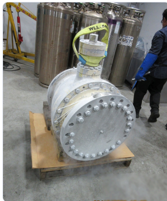
Cryogenic valve work in the Anthis shop, staged beside cryogenic test dewars.
