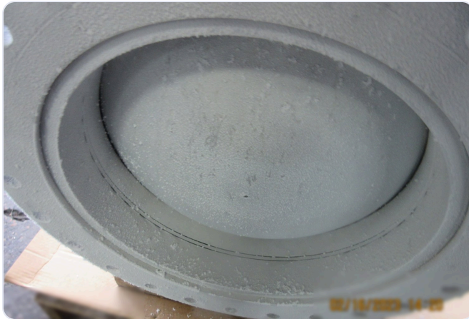
Inspection of the sealing face during teardown.
