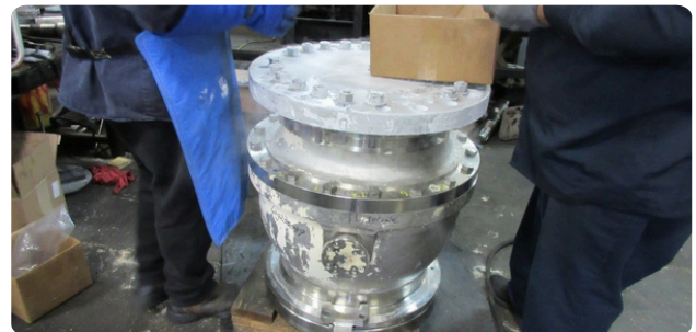
Reassembly and fit-up in the Anthis shop.
