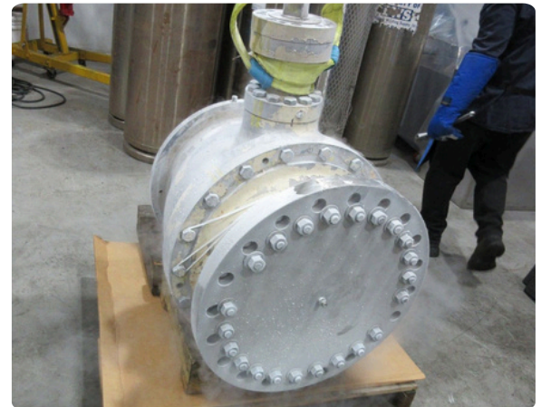
Cryogenic valve work in the Anthis shop, staged beside cryogenic test dewars.
