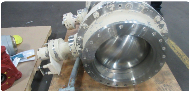
The rebuilt valve, bore and seat re-engineered and finished to a tight tolerance.
